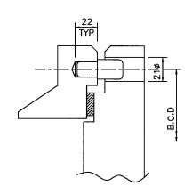
FIXING DETAIL OF DOWEL PINS
